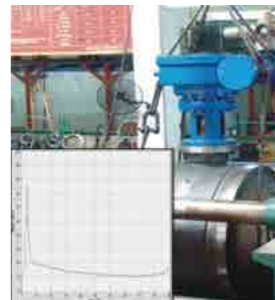
Valve Pressure Test and Full Travel Torque Test
