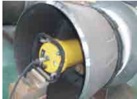
X-ray inspection of weld seam
