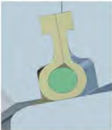
Valve closing medium flows from right to left The valve seat moves along the flow direction of the medium and is close to the butterfly plate to ensure the reliability of the bidirectional seal. It has reliable sealing performance from vacuum to high pressure.
