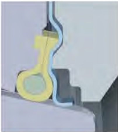
Fire Safety Seat Structure Under normal conditions, both the elastic seat and the metal seat of the seat assembly are in contact with the butterfly plate at the same time. In case of fire, when the elastic seat is partially or completely damaged, the metal seat always keeps stable contact with the butterfly plate. Reliable seals can be provided regardless of the flow direction of the medium.
